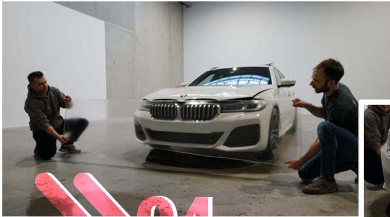
Place the Protector Ultra Top on the bodywork and stretch it to ensure it perfectly takes the surface's shape that needs to be covered
